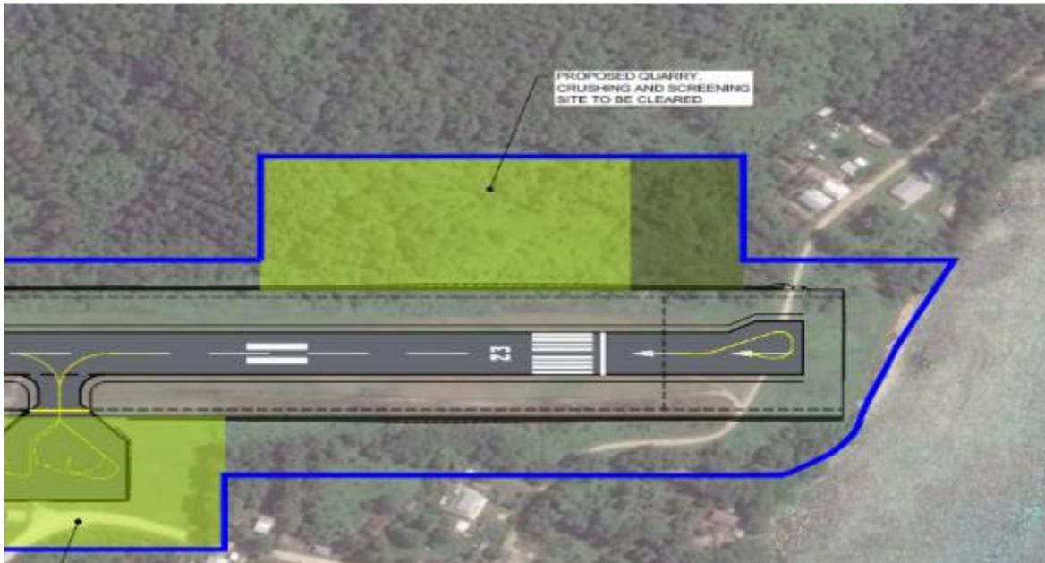
**Figure 8: Proposed site for project quarry (yellow) within the airfield lease boundary (approx. boundary shown in blue)**
